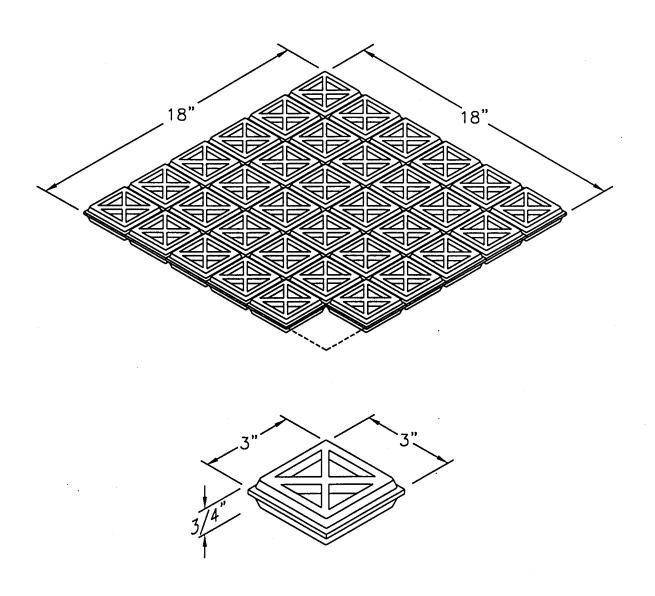
Type "400N" Neoprene Isolation Pad, offers an economical solution to reduce sound, shock and high frequency vibration transmitted by HVAC, industrial and process equipment. The "400N" pad is manufactured in blue oil resistant neoprene and is available in standard sheets of  $18" \times 18" \times 3/4"$ . Each sheet consists of  $(36) - 3" \times 3" \times 3/4"$  individual squares that can be easily cut with a utility knife.
