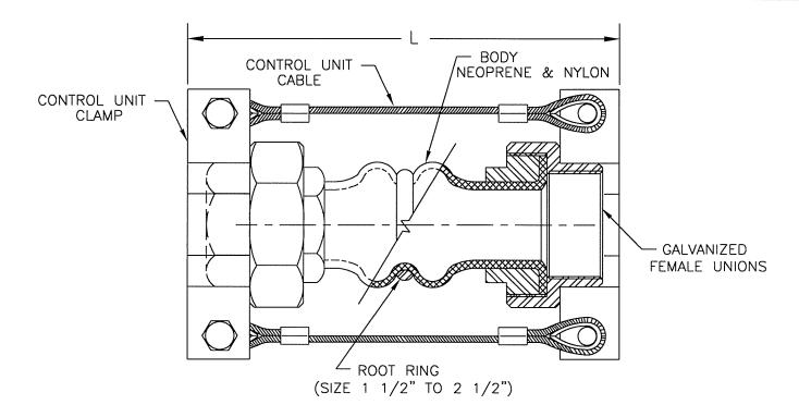
**Double Sphere Unions** are used for connecting pipes and equipment where threaded union ends are preferred. They are made of neoprene and nylon and are resistant to ozone and aging. They also accommodate thermal movement and misalignment.
